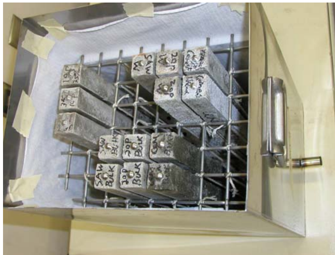
Figure 4-11 ASR bars cured in ASTM containers
