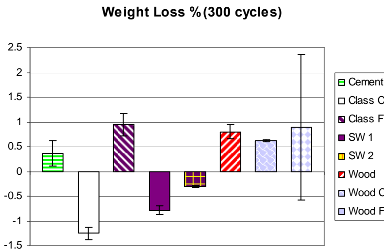
Figure 5-9 Freezing and thawing behavior of fly ash concrete samples
