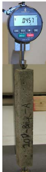
Figure 4-10 ASR bar length measurement (precision \pm 10^{-4} in)
